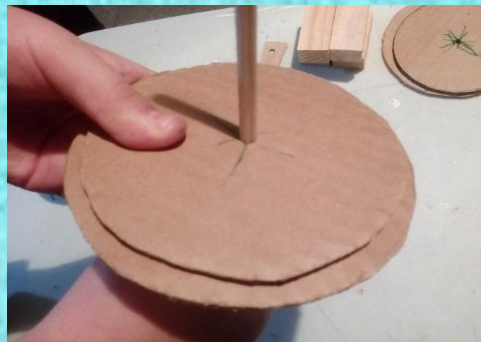
2. Make cardboard disks and pierce them through the center with a wooden stick.
